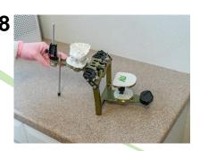
Open the articulator, remove the index tray and install the waxing spacer plate in place of the index tray.
