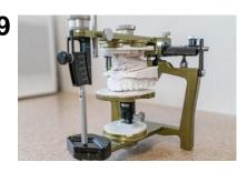
Determine the work needed (i.e. adding 2mm of incisal length). Unlock the table with the thumb screw, lower the table top by 2mm and lock in place with the thumb screw. Wax down to the table top
