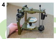
Place the platform securely on the magnetic base on the lower frame of the articulator.
