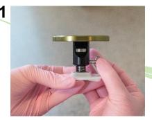
Unlock the platform with the thumb screw, use the thumb wheel to set the platform height to 0, and then lock in place with the thumb screw.
