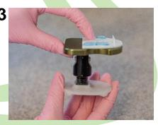
Snap the index tray onto the platform in the index holes, ensuring the tray is flat on the platform.
