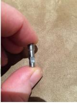
Using the 2.5mm hex screwdriver from your articulator, loosen the small allen screw in the mounting knob and remove the threaded insert. Note the notched section on the threaded insert
