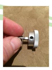
Locate the threaded insert back into the mounting knob, ensuring that the notched section is aligned with the allen screw. When ready, push insert all the way into the mounting knob and tighten allen screw to firmly hold threaded insert.
