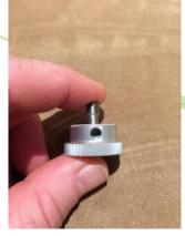
Remove mounting knob from articulator frame by unthreading it (counterclockwise). Note the small allen screw in the knob.
